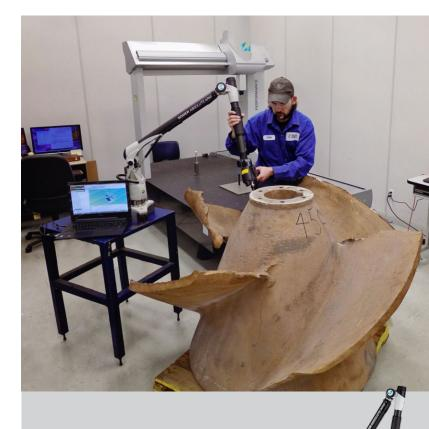
We can also reverse engineer existing castings or worn patterns with our portable 7 axis CMM with built in laser scanner, providing 2D & 3D data
